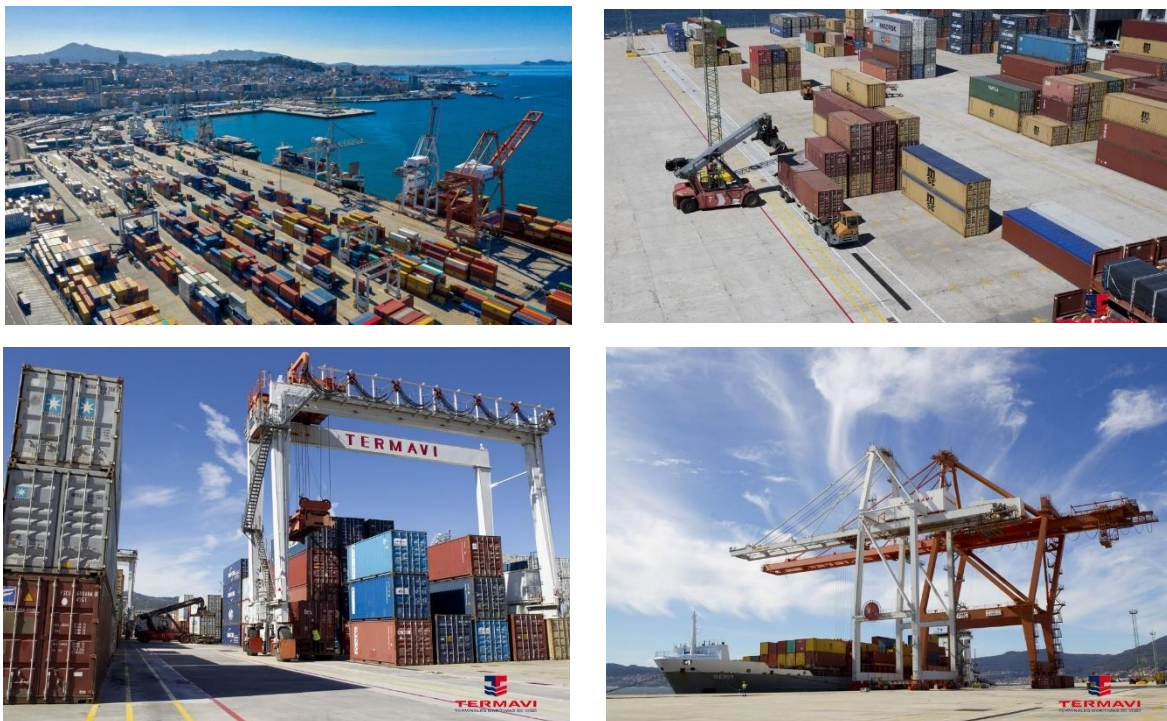
Figure 1: (From top left to right): 1) Vigo container terminal yard, 2) Reach stacker, 3) Rubber tyred gantry crane, 4) Quay cranes (Source: Termavi )
